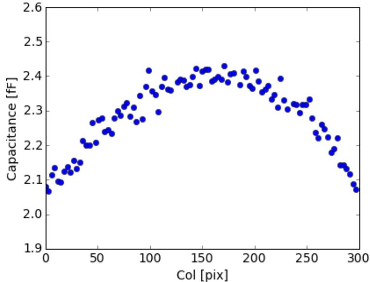
*Coupling capacitance between HVCMOS pixel pads and FEI4 amplifier pads have been measured (Bonn) along a pixel row of 1.5 cm length.*
