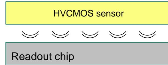
Capacitive coupled pixel detector - CCPD
