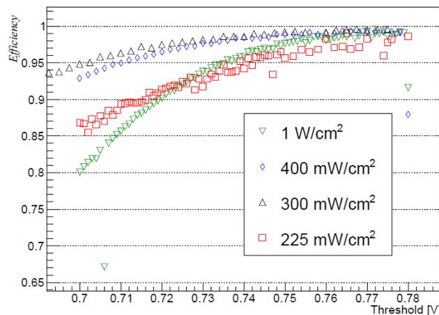
Efficiency as function of threshold for different power settings. Measured at PSI
