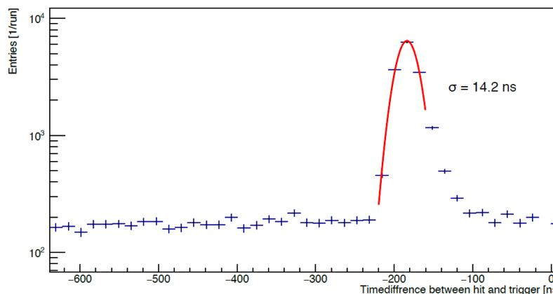
Timing resolution measured using settings with a power consumption of 300W/cm<sup>2</sup>. Shown is the difference in time between the hit in the DUT and the scintillators. Bin size is 16 ns. Measured at DESY
