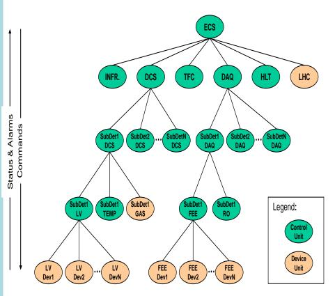
Control System (ECS) in LHCb is based on the SCADA WinCC OA with custom LHCb developed components.
