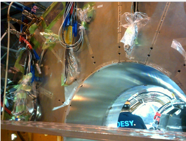
Detail of an endcap sector cable harness
