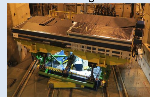
TileCal modules under test
