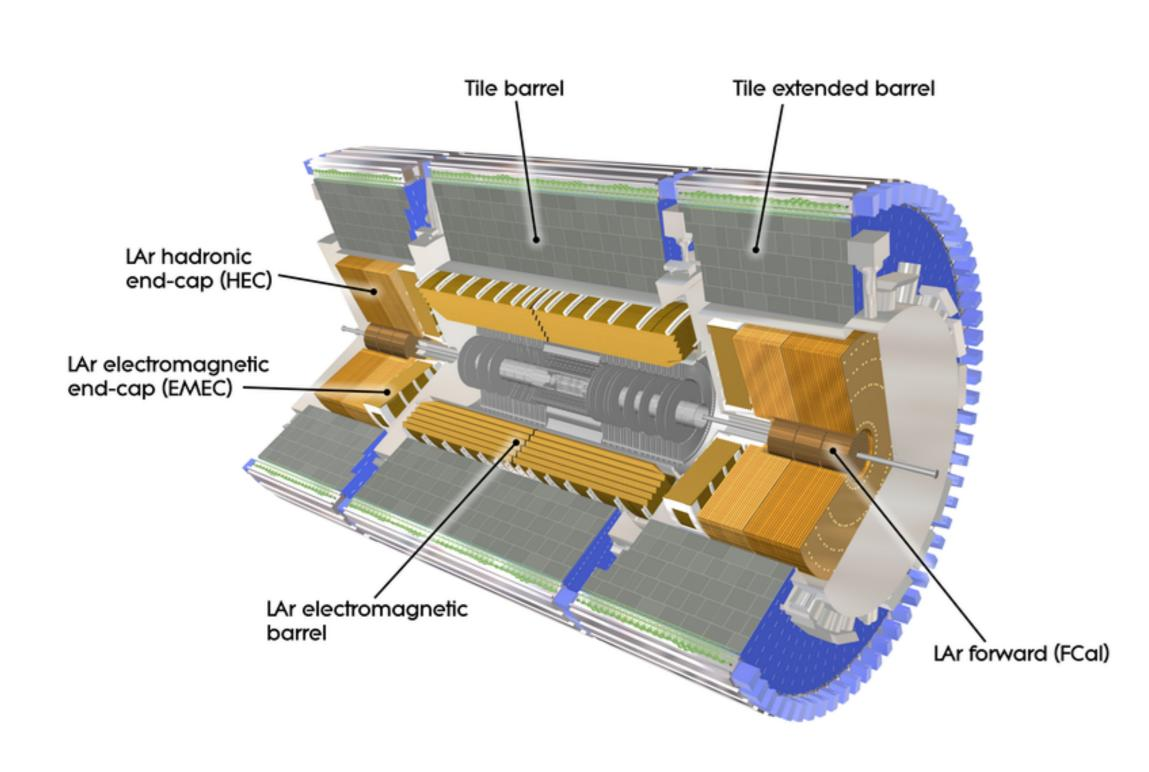
ATLAS [1] is one of the two large general-purpose detectors at the Large Hadron Collider (LHC) at CERN. The LHC started its operation in 2008 and since then it has gone through several gradual upgrades of beam energy and luminosity.
