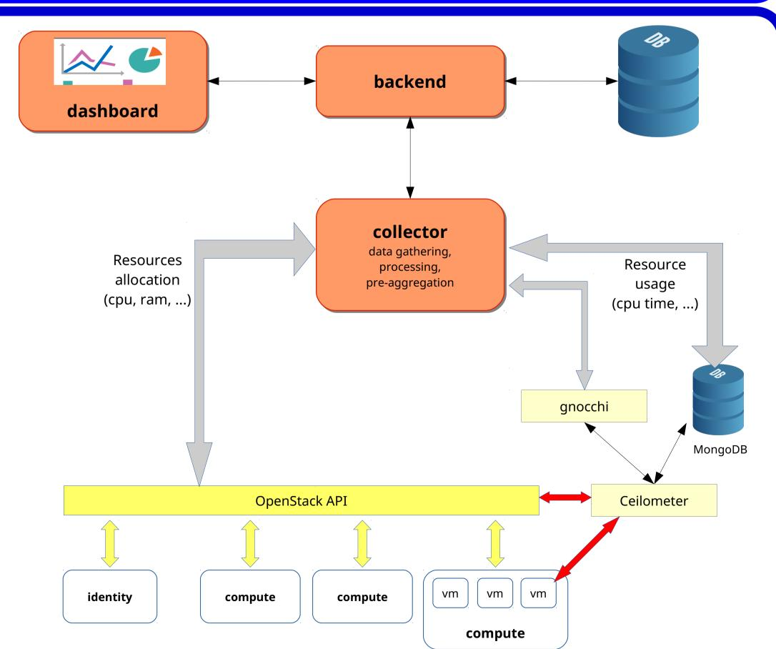
The collector gathers data at regular intervals from both the OpenStack API and the Ceilometer service. The data is then analyzed and pre-aggregated at coarser granularity (e.g. hourly), and metrics involving operations across different metrics are computed.
