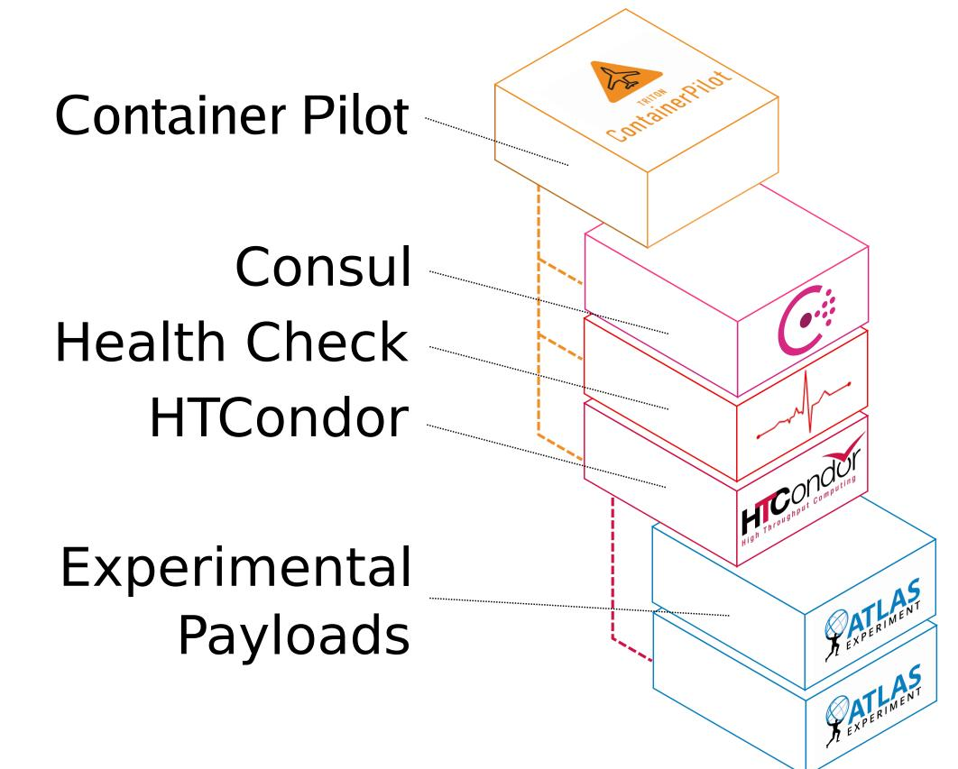
Container Copilot acts as an init system (similar to systemd) within the container itself. When a container is instantiated, its entrypoint is set to run the Container Copilot binary. This binary carries out a set of pre-configuration tasks and then runs and manages any jobs given to it. In our system, we use it to start both a Consul agent along with the HTCondor master daemon.
