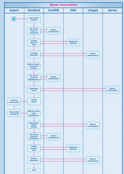
A typical workflow of actions performed while intervening on a server.
