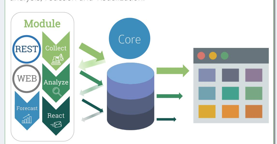
With this architecture it is possible to focus on modules: add and change them without affecting the whole system. This architecture also allow to implement modules which do not need to use any part of module, for example: it is possible to make a module which has only web and rest part, so it does not collect anything, but it can display on the web page data from monitoring database.
