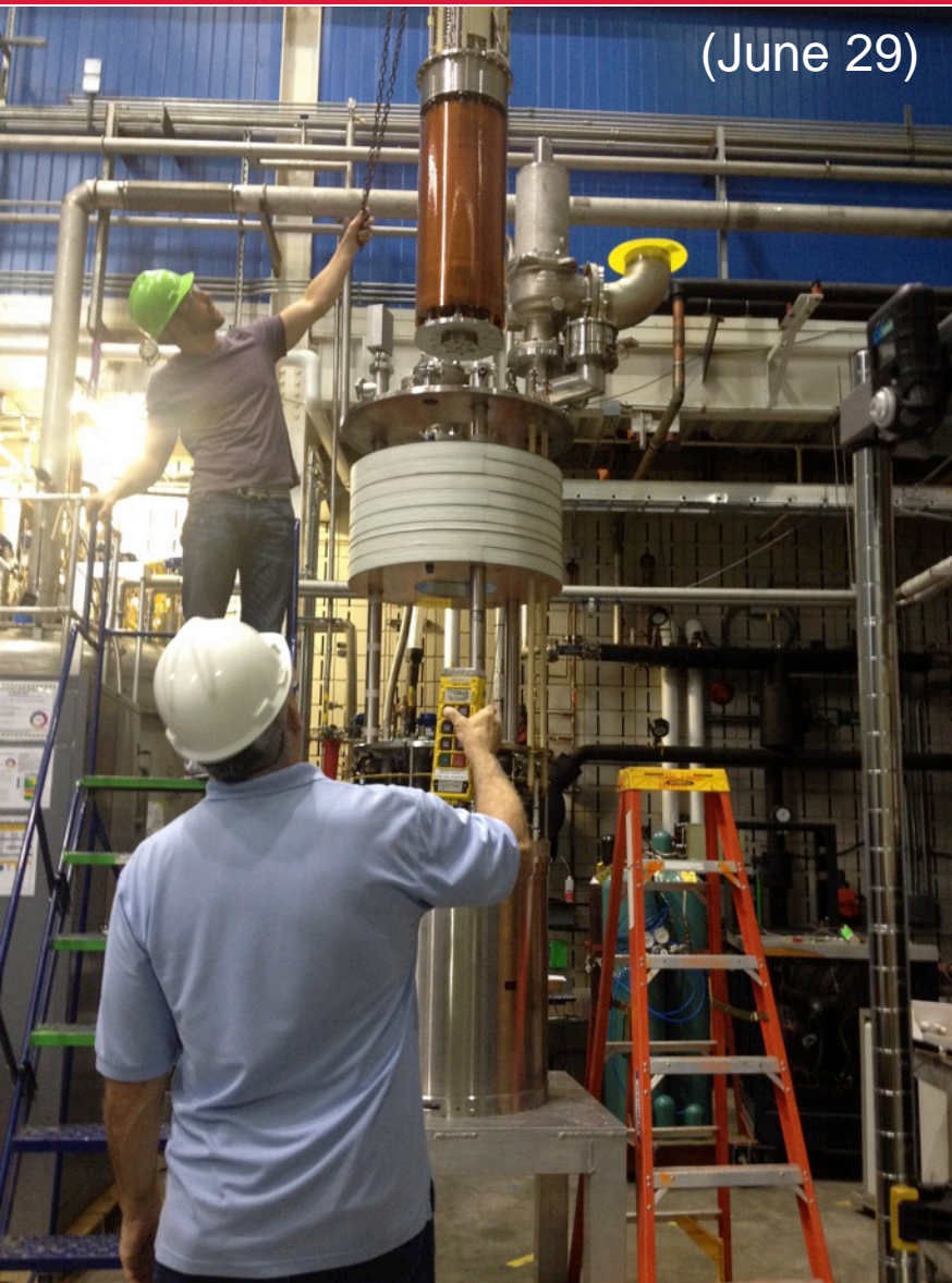
HTS assembly going into LTS magnet
