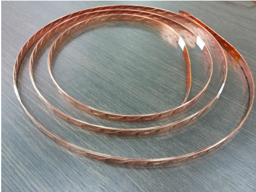
2.5 m PnC cable provided to CERN for testing
