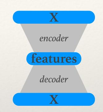
encoder and decoder: (stacks of) neural network layers
