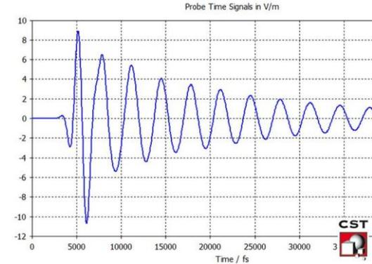
SRR shows a more resonant behaviour (not of interest, just need the slope around one zero crossing) and approx 30% higher amplitude, which should be more than compensated by factor 4 larger gap length of ISRR.
