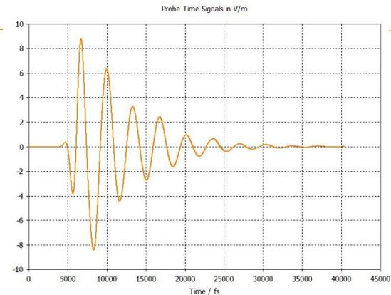
For comparison response of standard SRR design ( $f=0.3$  THz, 20  $\mu\text{m}$  thickness)
