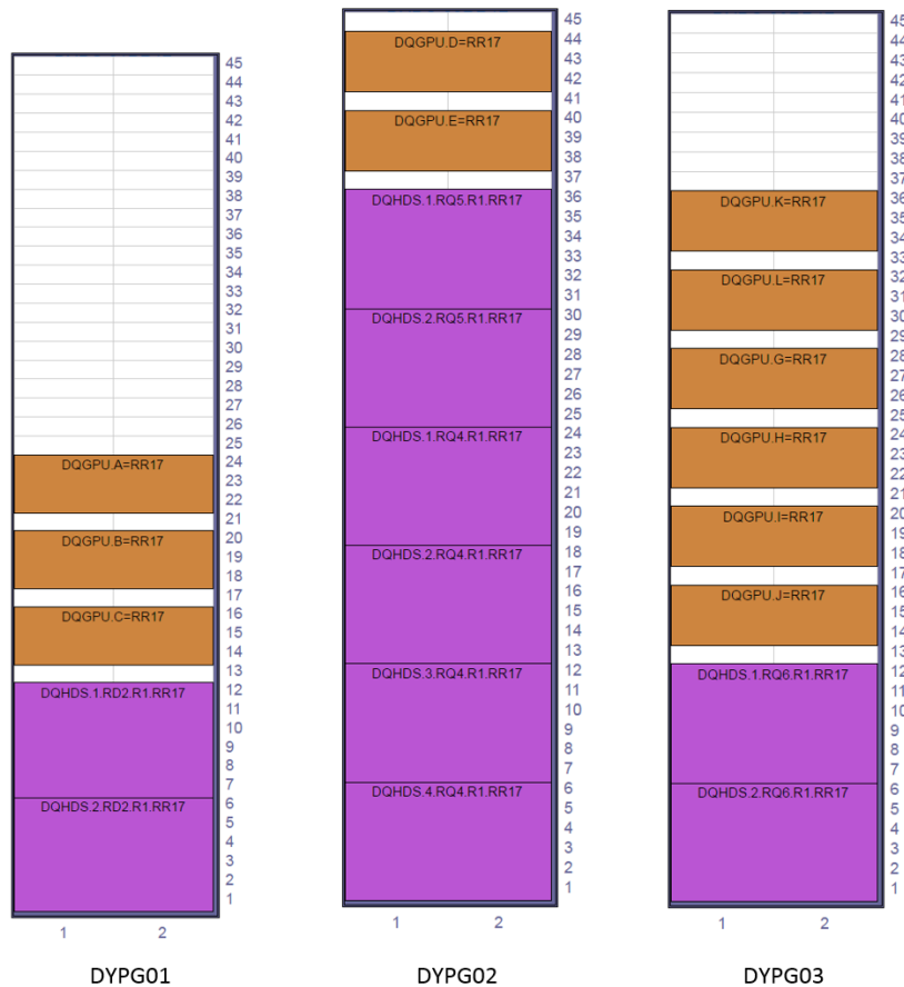
Figure 6: LHC QPS racks for DQHDS in RR17
