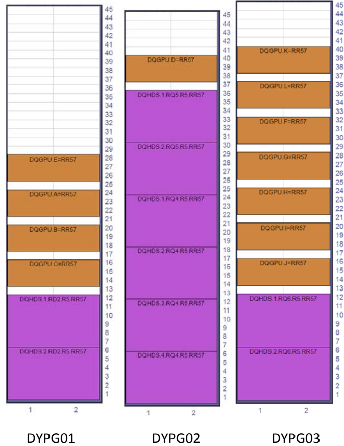
Figure 11: LHC QPS racks for DQHDS in RR57
