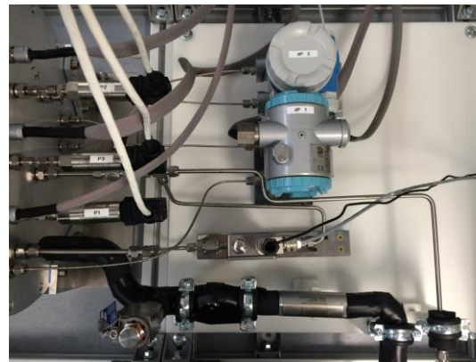
Differential & absolute pressure sensors and flow meter outside the vacuum vessel
