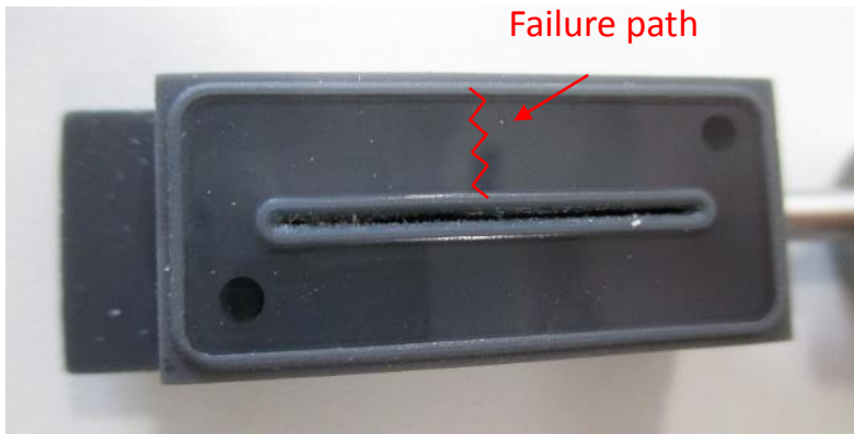
Connector after pressure test
