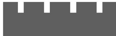
trenches - anisotropic etch
