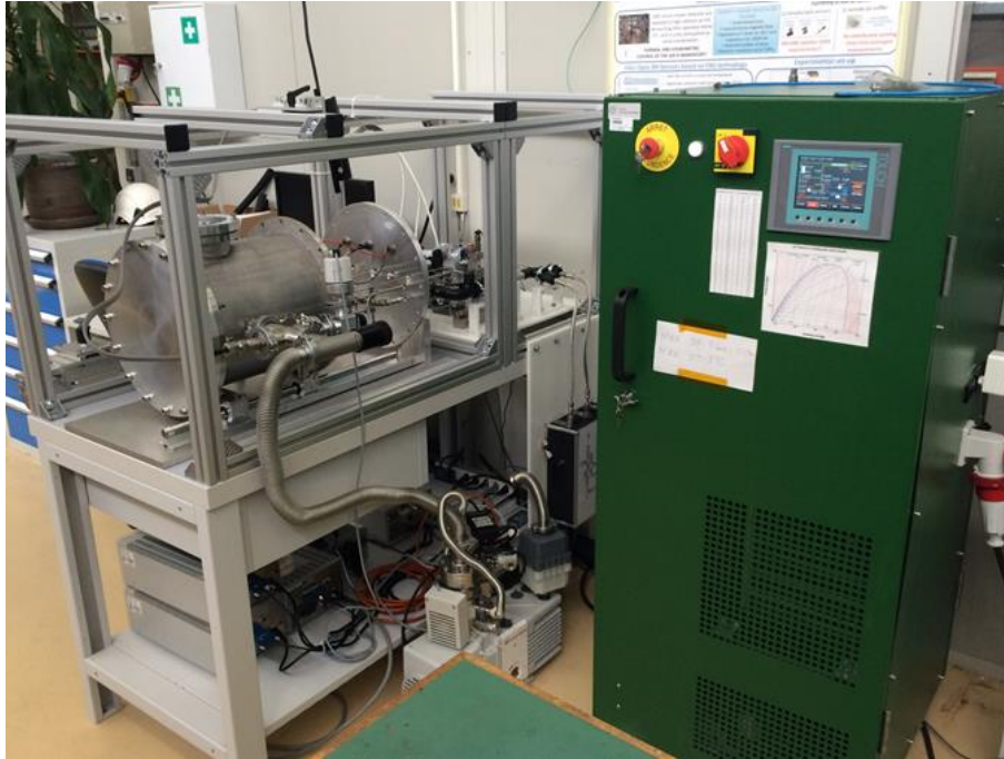
Fig. 7 New test facility for evaporative CO 2 flow measurements in mini- and micro-channels (I)
