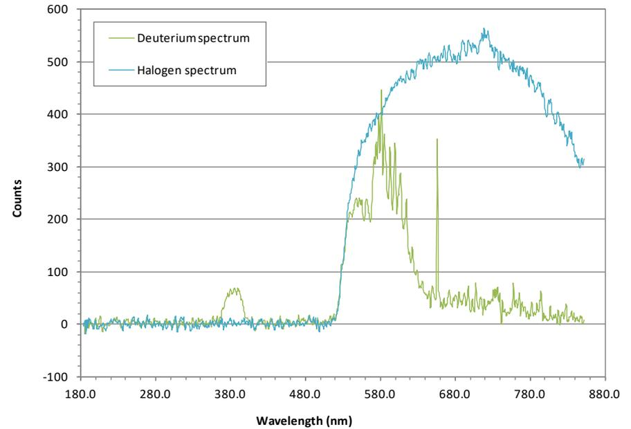
(Note that the 'bump' in the background signal level is due to the longer fibre channelling ambient light)
