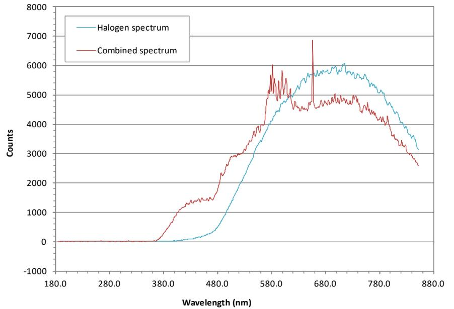
(Note that the three 'spikes' in the background signal are fixed pattern noise from the spectrometer)
