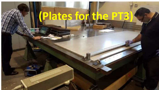
Measurements using laser interferometer. Over a flat table (~0.1mm planarity)
