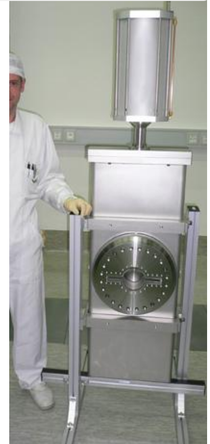
Gate valve for beam pipes with antechambers
