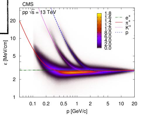
Identified from the energy deposited in the silicon tracker and the reconstructed particle trajectory.
