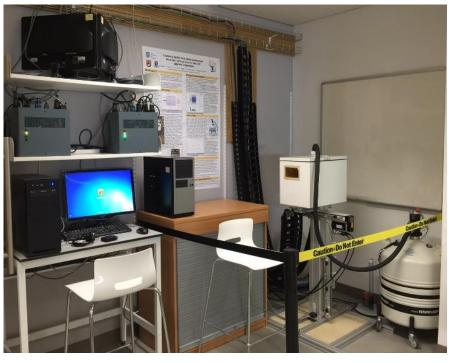
To test and implement upgrades to the scanning system and software, a second scanning system and LN2 cooling unit is undergoing installation in <a href="Sheffield Robotics">Sheffield Robotics</a>. Sited in the 300m<sup>2</sup> Robotics Foundry in the new purpose built 7 story, 5355m<sup>2</sup> Pam Liversidge Building for "Interdisciplinary Research".
