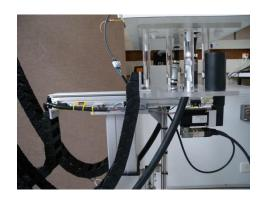
Overall unit length with a parallel mounted motor is 598mm long to reduce working space
