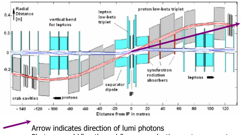
Photons would "go through" superconducting proton magnet
