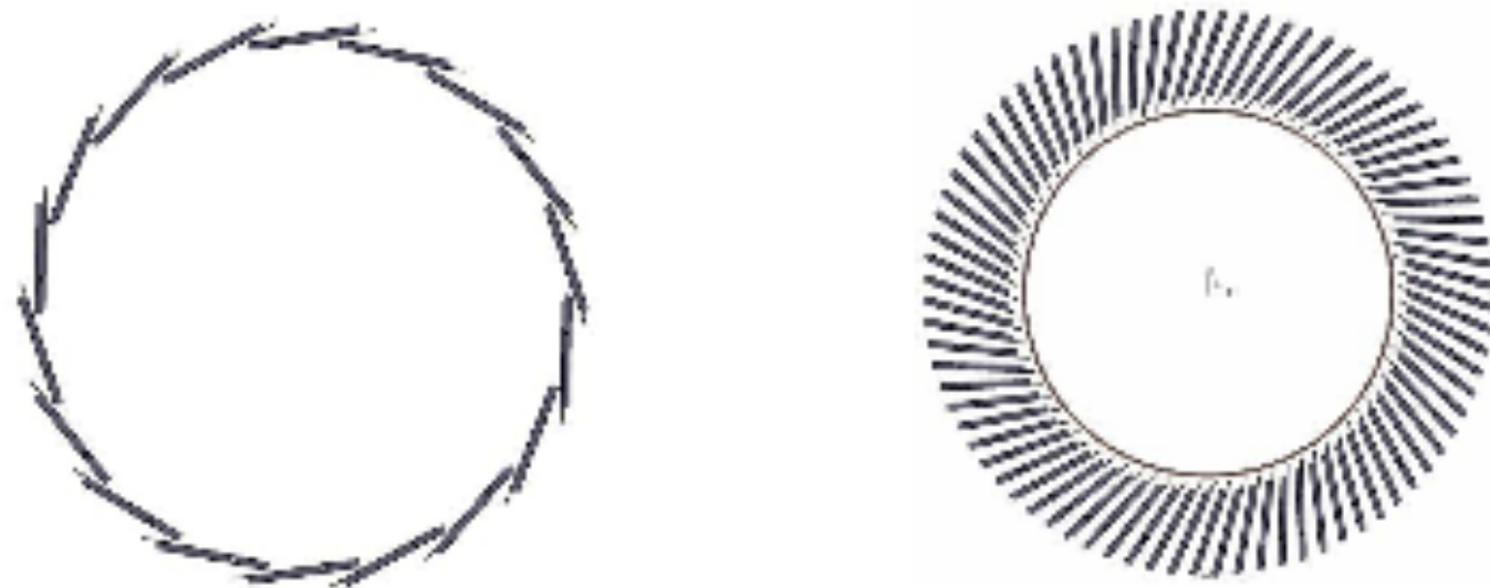
Fig. 25. Left: a layer of Gossip detectors with the angle of incidence equal ( \pm 0.1 rad) to the Lorentz angle for stiff tracks. Right: in case of sufficient time resolution, the spatial (4D!) resolution of Gossip is independent of the incident track angle, allowing a larger range ( \pm 0.8 rad) of the angle of incidence.
