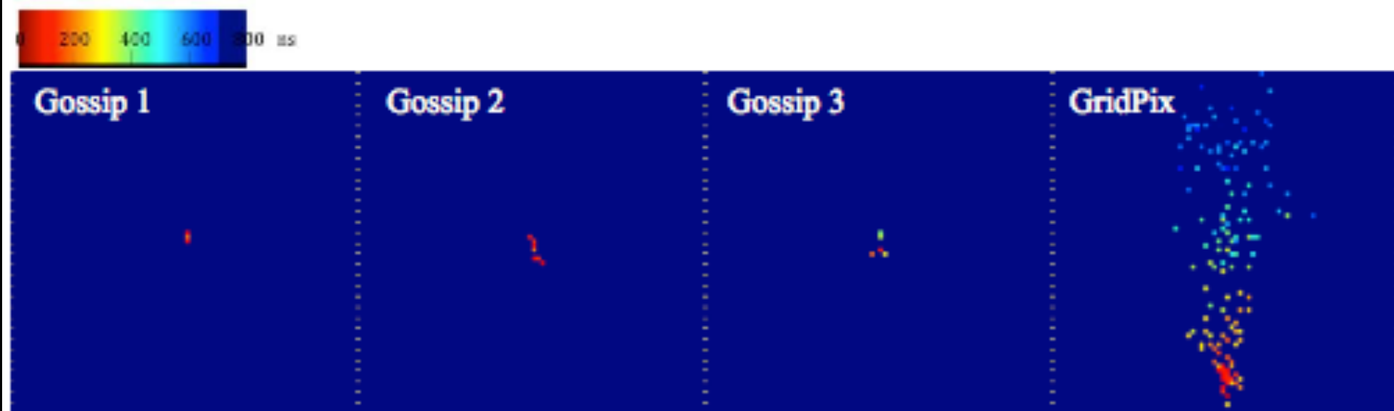
Fig. 11. Drift time plots of a typical event from a 15 GeV \pi^- traversing three Gossip prototypes and a GridPix detector with 20 mm drift height. The drift times are indicated by colours. For better visibility only a rectangle of 80*80 pixels is displayed of each detector.
