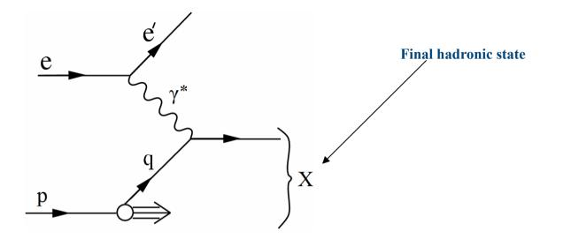
Feynman Diagram of a General Deep Inelastic Scattering Process ( $ep \rightarrow e' X$ )
