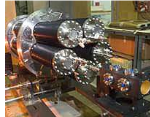
CNGS target design average beam power: 750 kW
