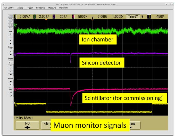
Neutrino production is confirmed by associated muon signal
