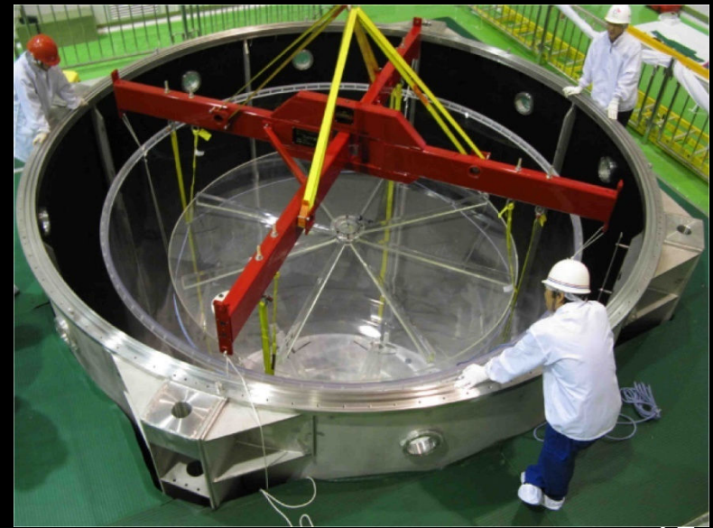
Detector mechanics: 5-m SST vessel, 4-m and 3-m acrylic vessels in assembly hall
