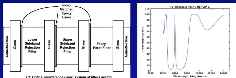
Blocking filters are required to suppress the unwanted light transmission in the side lobes on either side of the band-pass. These filters can be constructed using either absorbing or interference based approaches. However, advantage can be obtained in suppressing the off-band transmission by adding a thin metal layer to act as the cavity known as an induced transmission filter. Multilayer metal filters can also be realized which will improve suppression on the long wavelength side.
