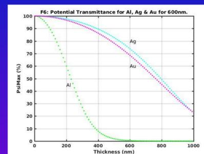
The Maximum Potential Transmittance for each metal can be calculated over a range of metal thickness and wavelengths (F5). By selecting a particular wavelength the range of available transmittances are shown (F6). The optical admittance of the metal layer for the thickness and central wavelength values is used to design the dielectric stack which must include a non 1/4 wavelength layer on either side to make the complex index of refraction 'real' to match the substrate.
