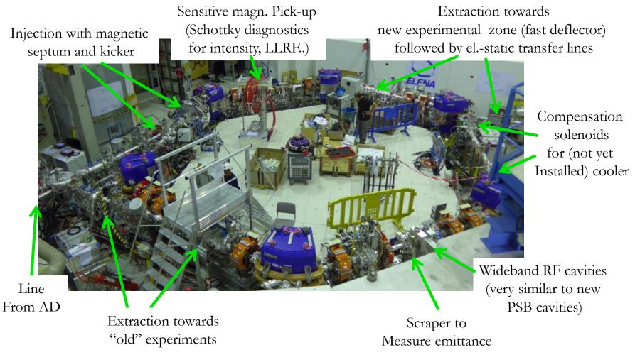
Short 30.4 circumference Ring, Challenges due to low (100 keV) Energy and Intensity (low magnetic Fields, Rest Gas Interactions, Beam Instrumentation with weak Signals
