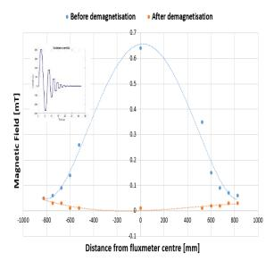
Degaussing reduces the the integrated remanent field from 153 to 0.03 mTm.
