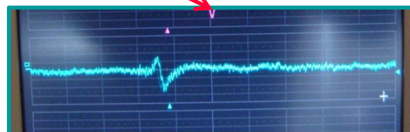
Trigger Signal with rise and decay time reshaped
