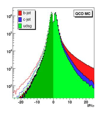
The Impact Parameter of a track is positive (negative) if angle θ between the IP direction and the jet axis is smaller (larger) than 90°
