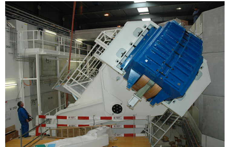
Final dipole of Gantry 2 at PSI. Large 45-tonne final dipole
