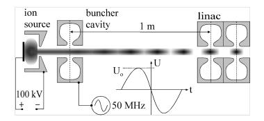
Question: What's the required voltage amplitude  $U_0$  of the buncher cavity? Hints:
