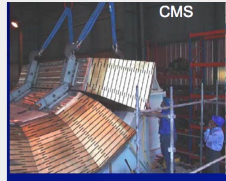
5 cm brass / 3.7 cm scint. Embedded fibres, HPD readout
