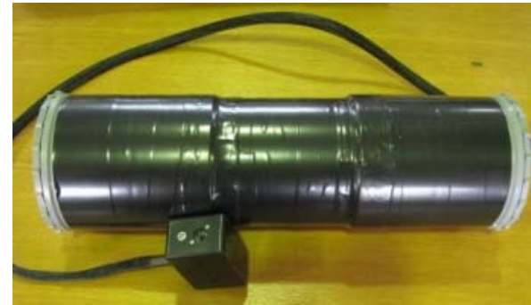
A scintillator to measure the muon lifetime
