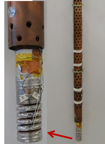
Walters' Spring probe for strain sensitivity studies of I_c in SC wires
