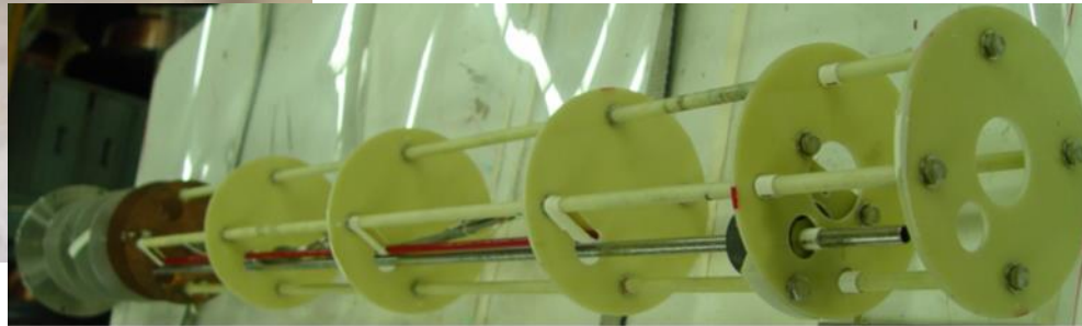
New Hall probe system to measure shielding of bulk MgB_2 tubes
