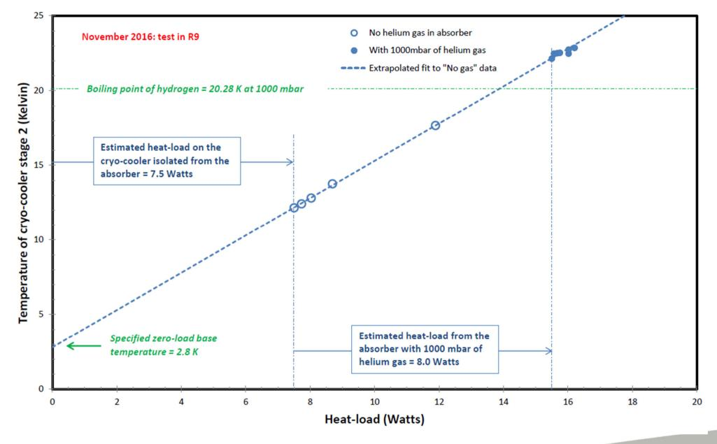
To cool the system to liquefy hydrogen, we need to reduce both the heat load through the turret and the heat load from the absorber.
