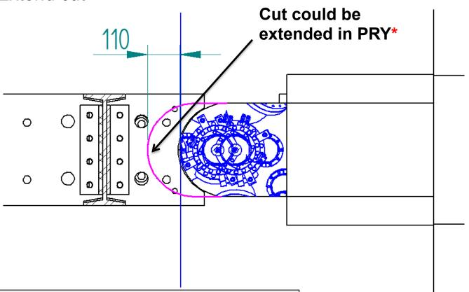
Putting back in 30 mm clearance the RF device could be moved a further ~ 80 mm
