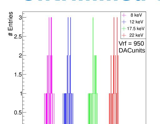
The threshold dispersion is given by the spread of the inflection points, i.e. the resulting thresholds, over all sensor-strips.
