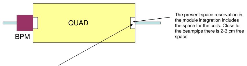
Small window frame magnet or a variant with magnetic shielding towards the quad can go into that free space.
