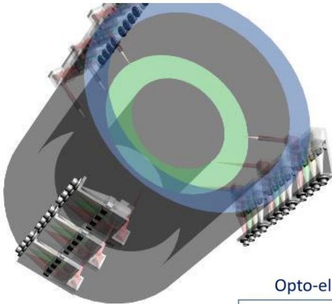
The  $\Delta d$  is measured with a heterodyne interferometer ( $\times 9$  optical heads) with picometer resolution
