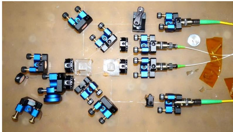
1 pm/ $\sqrt{\text{Hz}}$  @ 1 Hz has been demonstrated with a breadboard based on a 1  $\mu\text{m}$  free running laser
