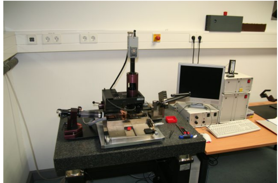
Finetech Lambda, 1 \mu m precision, 400°C, 20K/s, 200N
