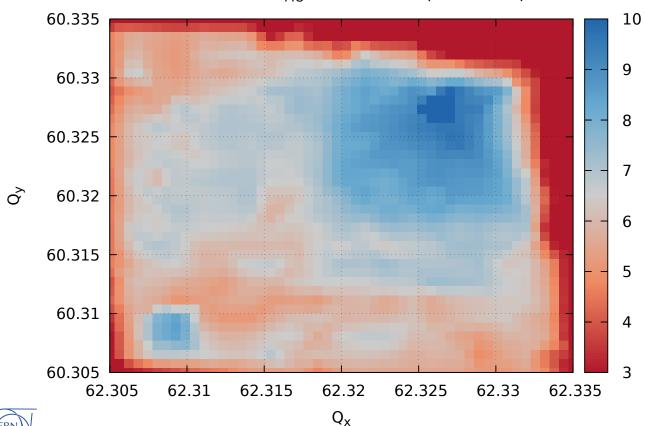
HL-LHC v.1.2 - Min DA; Q'=3; I<sub>MO</sub>=-570 A;  $\epsilon$ =2.5 µm; X=255 µrad; LHCb on
