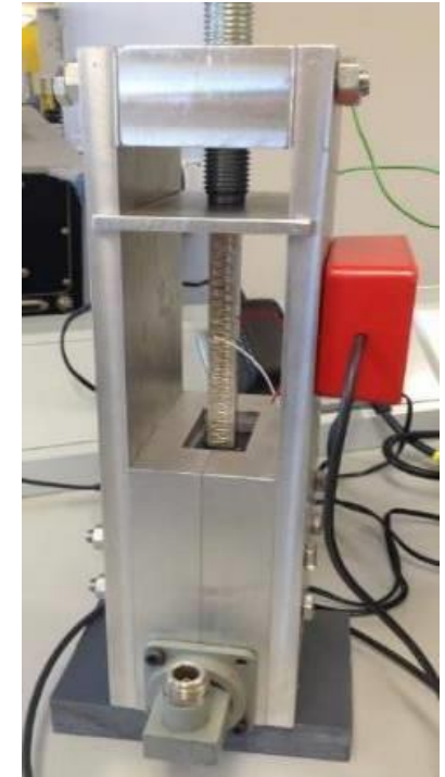
Prototype high power phase shifter built at Lancaster university, being used for current testing
