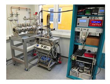
Works concentrated on the primary cathode – an experimantal setup for evaporation and diagnostics of CsK<sub>2</sub>Sb photocathodes has been established
