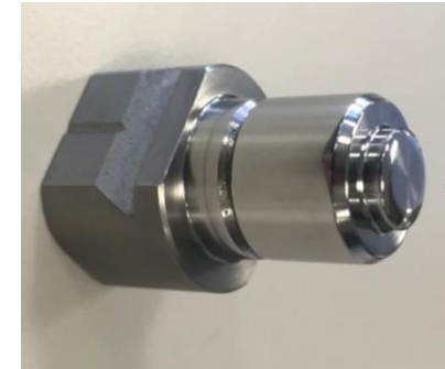
Mo photocathode plug of the HRRG
