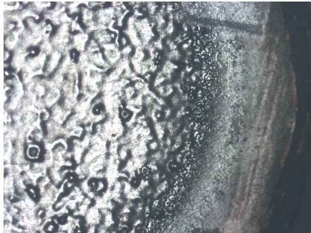
optical microscope view of deposited Pb layer
