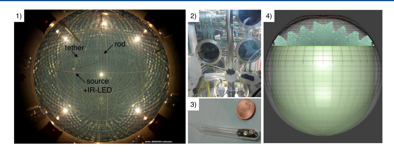
large volume, liquid scintillator (PC+PPO) detector and its primary purpose is the real-time measurement of low-energy solar neutrinos [2]. Its unique properties make it also suitable for the investigation of a possible sterile neutrino state in the SOX experiment [3].
